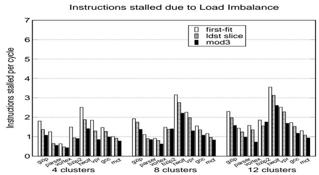
Fig. 4. Average Number of Instructions Stalled per Cycle; Fetch size = 16, Cluster issue width = 2, Cluster window size = 16, **Interconnect = Crossbar**
