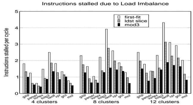
Fig. 5. Average Number of Instructions Stalled per Cycle; Fetch size = 16, Cluster issue width = 2, Cluster window size = 16, **Interconnect = Bi-directional Ring**
